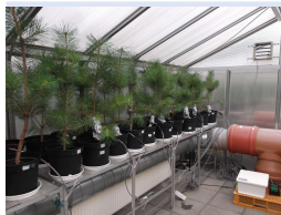
Figure 1: Pine seedlings in ventilated greenhouse. Filtered air (FA) or unfiltered, ambient air (AA) was introduced from the tubing in the rear and below the tables.
