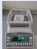
Figure 2: g_{min} determination of pine needles by drying curves
